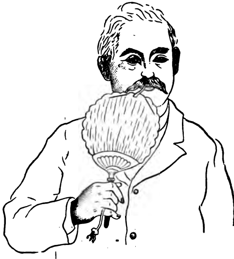
FIG. 29.—THE AUDIPHONE APPLIED.
